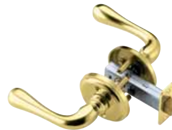
U.S. Lever Latch set. Handle model Diamond. Rose type TB. Screws visible on inside. 2 3/4 or 2 3/8 backset passage function. 2 3/4 or 2 3/8 backset privacy function.
