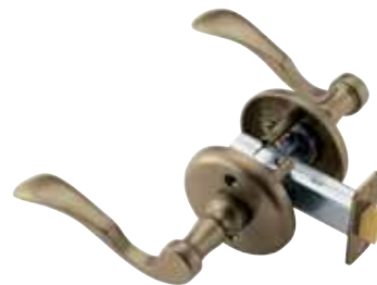
U.S. Lever Latch set. Handle model Alsace. Rose type BB. Screws visible on inside. 2 3/4 or 2 3/8 backset passage function. 2 3/4 or 2 3/8 backset privacy function.
